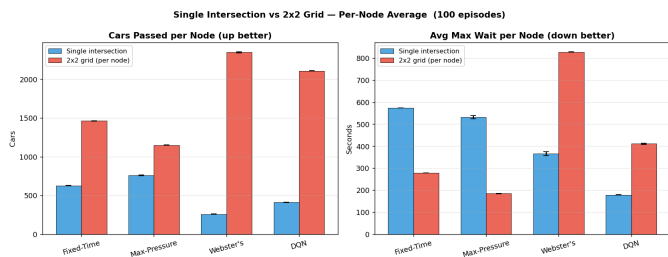
Fig. 9. Per-node average performance on the 2 \times 2 grid compared to single-intersection results.
